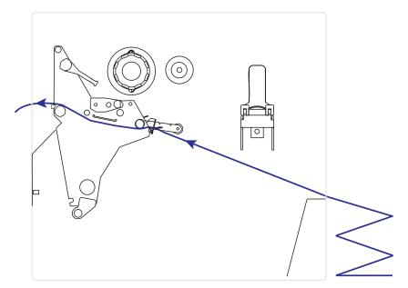
Figure 16 • Rear Feed Using Media Supply Hanger
